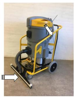
The airflow is drawn through the HEPA-filter, which will hold back the very fine dust particles.
