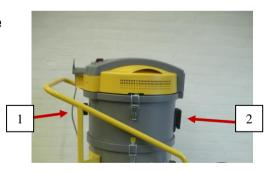
In this way you can read on the vacuum indicator whether the multi-tube filter is blocked and needs a cleaning. The cleaning is made by means of the pressure equalization valve.
