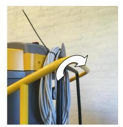
It is possible to lift the front nozzle from the floor by pulling the handle near the steering grip.
