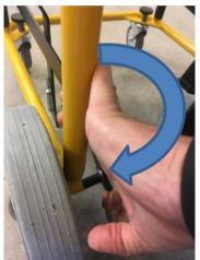
Pull the lifting handel at the steering grip -
