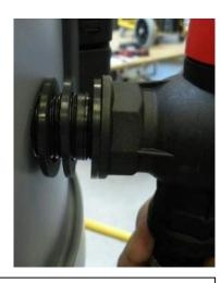
In the adaptor ring a pilot drilling is marked where the  $\emptyset$ 26 mm hole is to be bored. Mount the 3-way valve with the 3 washers enclosed on the outside and the nut on the inside.
