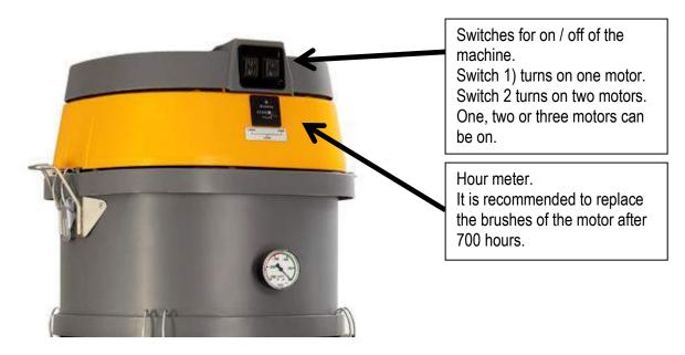
The three motors (3300 W): One switch turns on two suction motors, and the other switch turns on the third motor.
