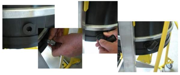
Unscrew the blind plug and mount the hose connector with the washers enclosed.
