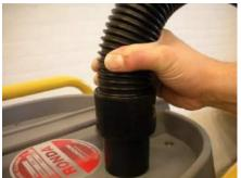
Pull the flap of the shock valve (a regular pull, not a tug)
