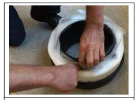
Pull the part of the bag that was put down into the centre of the dispenser over the rubber band
