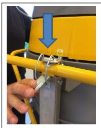
During transport the transport bracket / handle MUST be locked.
