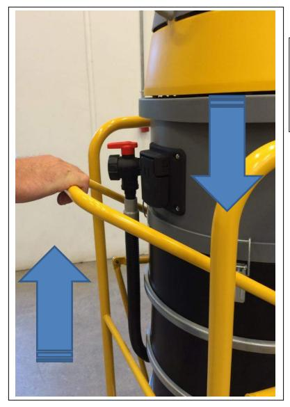
The machine is transported standing. You can lower the machine to transport position by using the handle in front
