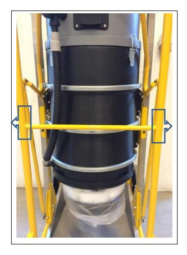
The machine is transported standing. Clamping etc. only round the cross bar at the front of the frame.
