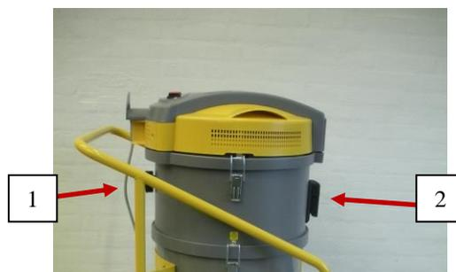
In this way you can read on the vacuum indicator whether the multi-tube filter is blocked and needs a cleaning. The cleaning is made by means of the pressure equalization valve. Also see the section about filter cleaning during operation.
