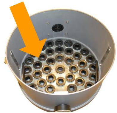
If the multi-tube filter is damaged, or if there are holes in surface of the filter, the multi-tube filter must be replaced. If the multi-tube filter is replaced, the HEPA-filter should be replaced at the same time. See the next page.
