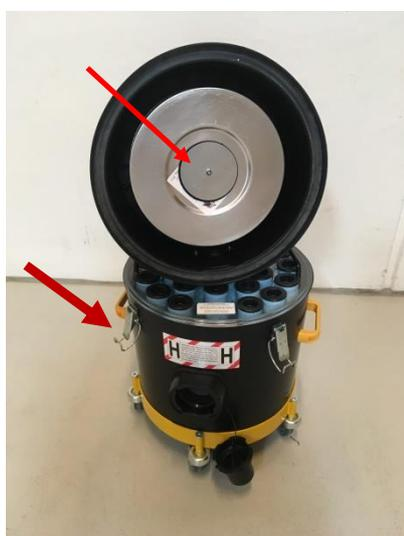
Loosen the four container clips of the motor top and remove the motor top. Place the motor top so that the filter is easily accessible.
