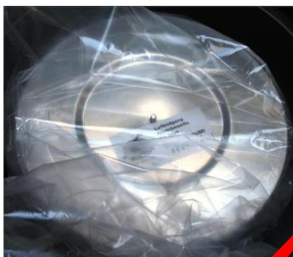
Pull a plastic bag (100 µm or the like) over the filter.
