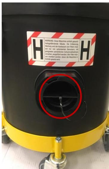
The container is equipped with a plug which is to be used during transport and whenever the machine is not operating.
